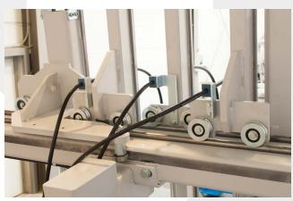
clamping beams on sliding rails for easy manipulation
