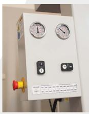
Two pressure gauges for vertical and horizontal direction
