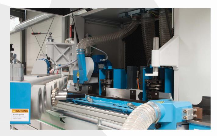
Profiling machine for comlete moulding of timbers in one single operation
