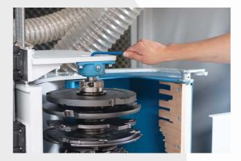
release shaft bearing using allen key
