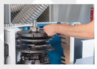
release hydro nut using allen key
