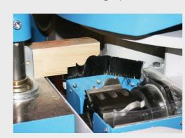
Horizontal milling unit for heritage sash horn detail or trenching of sash box (optional)
