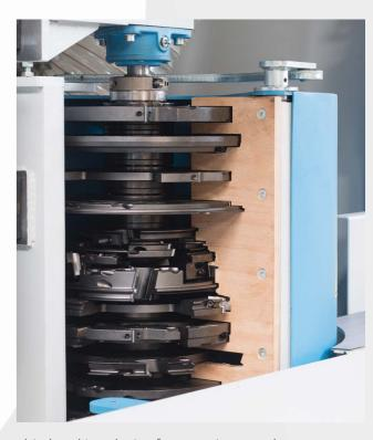
chip breaking device for tenoning matches the tooling stack
