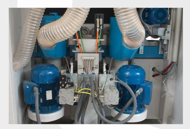
First class linear bearings for all linear guides on moving parts Servodrives for quick and precise setup of units
