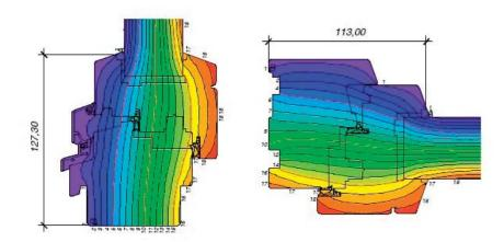
Simulation IV92 acc ISO 10077/2 and 10077/1 - value of frame Uf=0,94 and with aluminium waterbar Uf=1,10 W/m2°K  $Uw = 0.89 \text{ W/m}^2\text{°K}$  with Ug= 0,7 W/m²°K with TGI/Termix spacers (soft wood)
