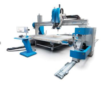
A complete production line for prefabricated wooden buildings designed according to the production requirements. Cutting and milling of structural elements, assembling on workbenches, panel handling and complete CNC bridge machining. Import of working data in BTL format and CAM control by Lignocam.
