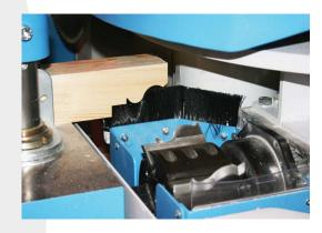
Horizontal milling unit for horns and trenching operations
